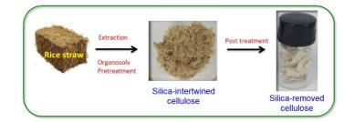
A one-pot process for the selective removal of silica from rice straw
